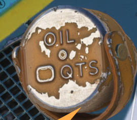
OIL CAP Use tablet to open oil cap to check the oil level
