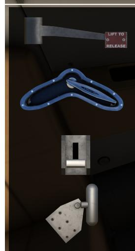
**UPPER DOOR HANDLE:** The upper handle will un-latch the upper section of the door. To un-latch the motor hook must be un-hooked. To latch the upper door handle, the motor hooks must be hooked. The motor hooks must be motored back to the un-hooked position after the door is latched otherwise the red DOOR annunciator will illuminate.
