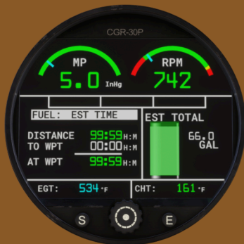
Estimated Time: Displays estimated flight time and time remaining to the selected waypoint/destination.
