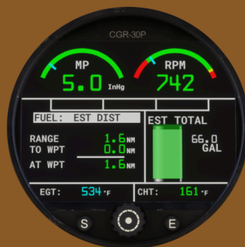
Estimated Distance: Displays estimated fuel range and distance to the selected waypoint/destination.
